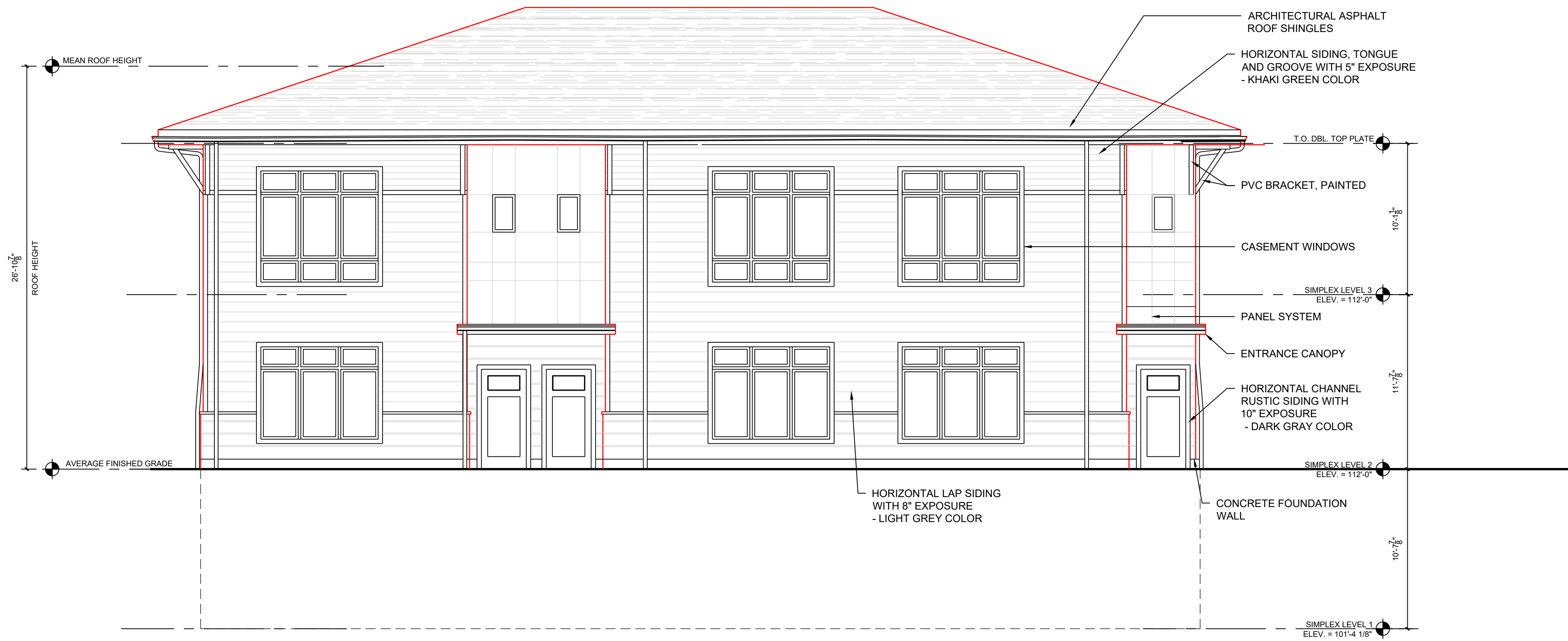
1 STATION EAST ELEVATION 3/16" = 1'-0"
