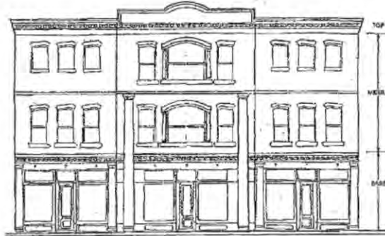
Figure 1: Use projecting cornice features and more detailed architectural elements on the first floor to create architectural variety on building facades.
