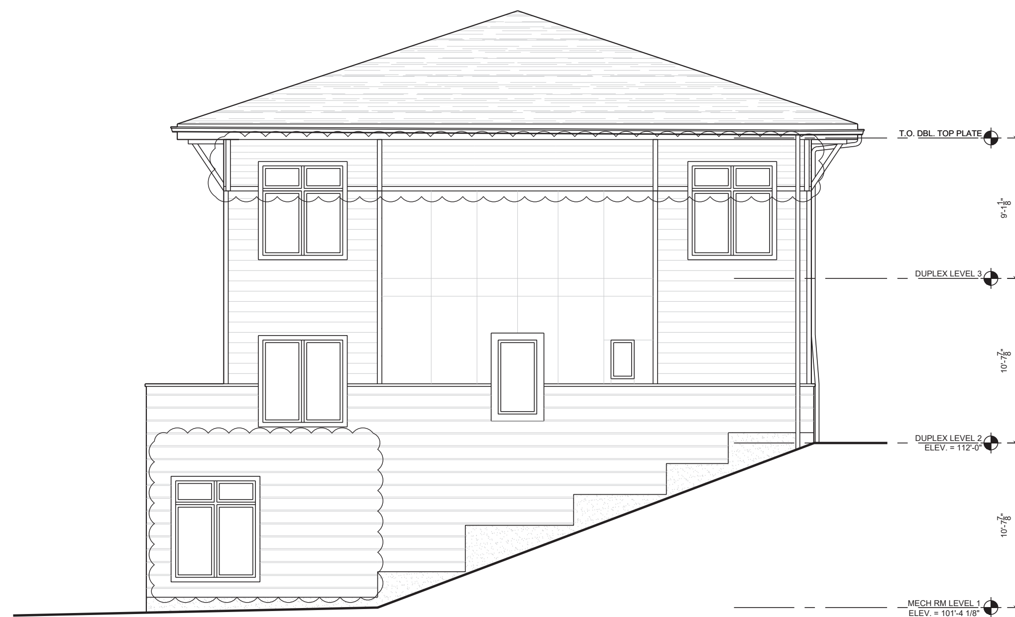
3 RIVER SOUTH ELEVATION 3/16" = 1'-0"
