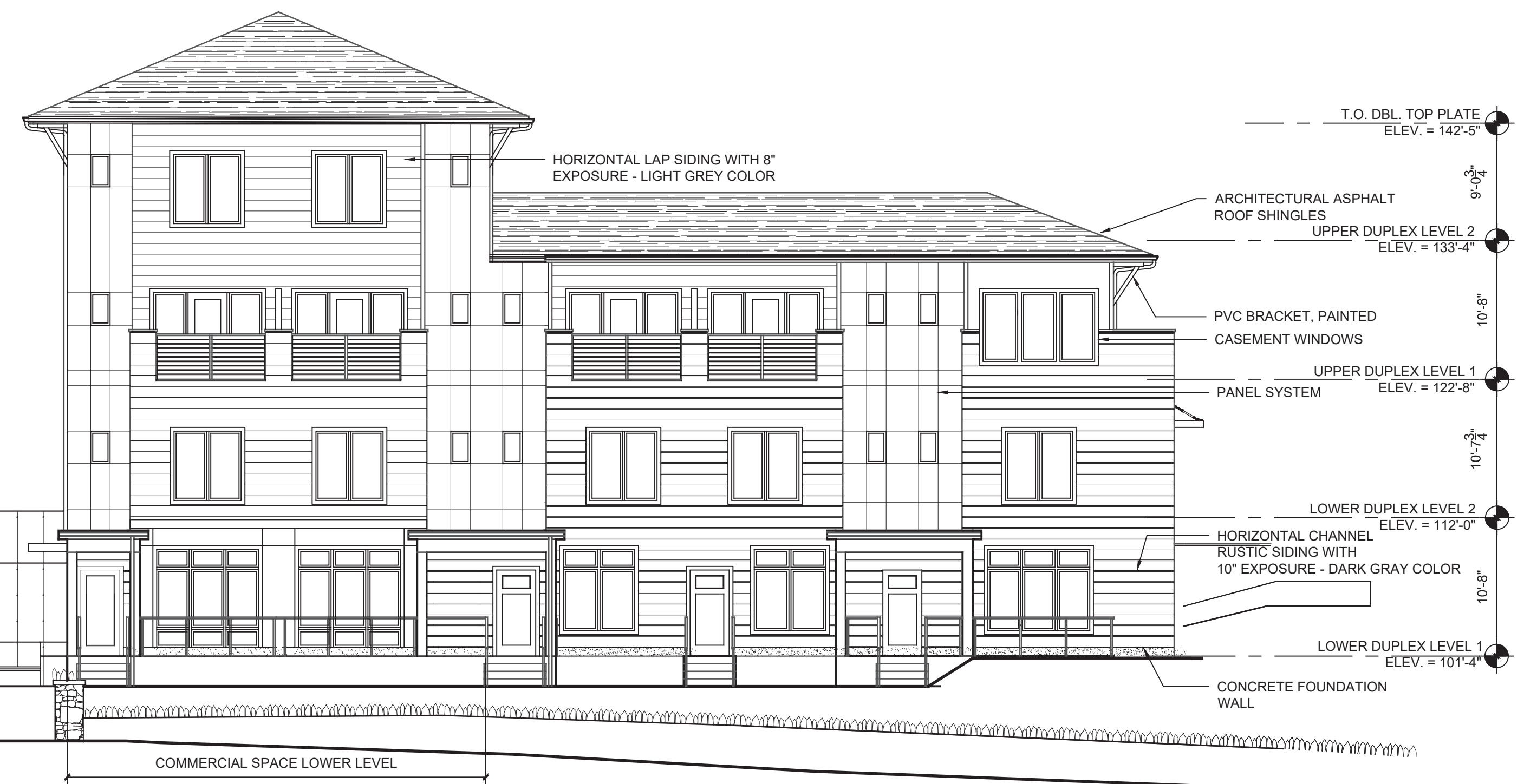
2 DONGAN BUILDING - NORTH ELEVATION (PROPOSED) 1/8" = 1'-0"
