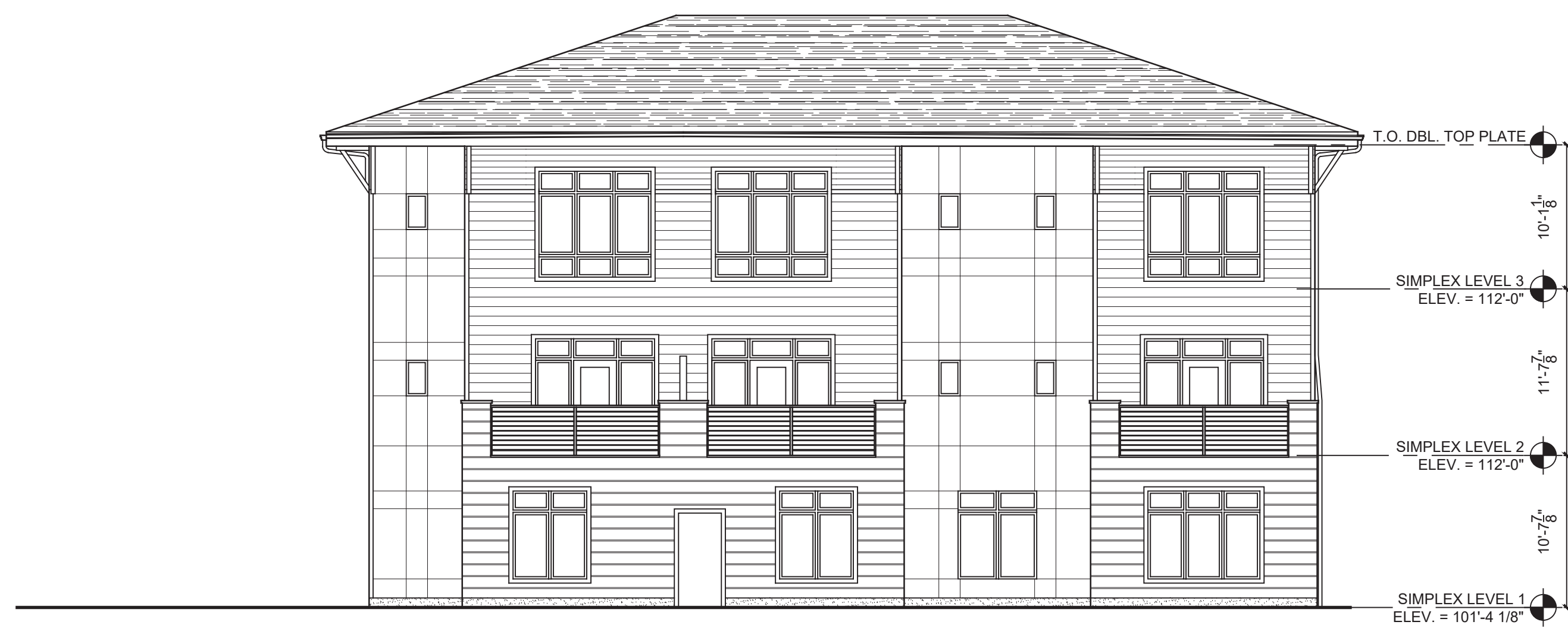
4 STATION BUILDING - WEST ELEVATION (PROPOSED) 1/8" = 1'-0"
