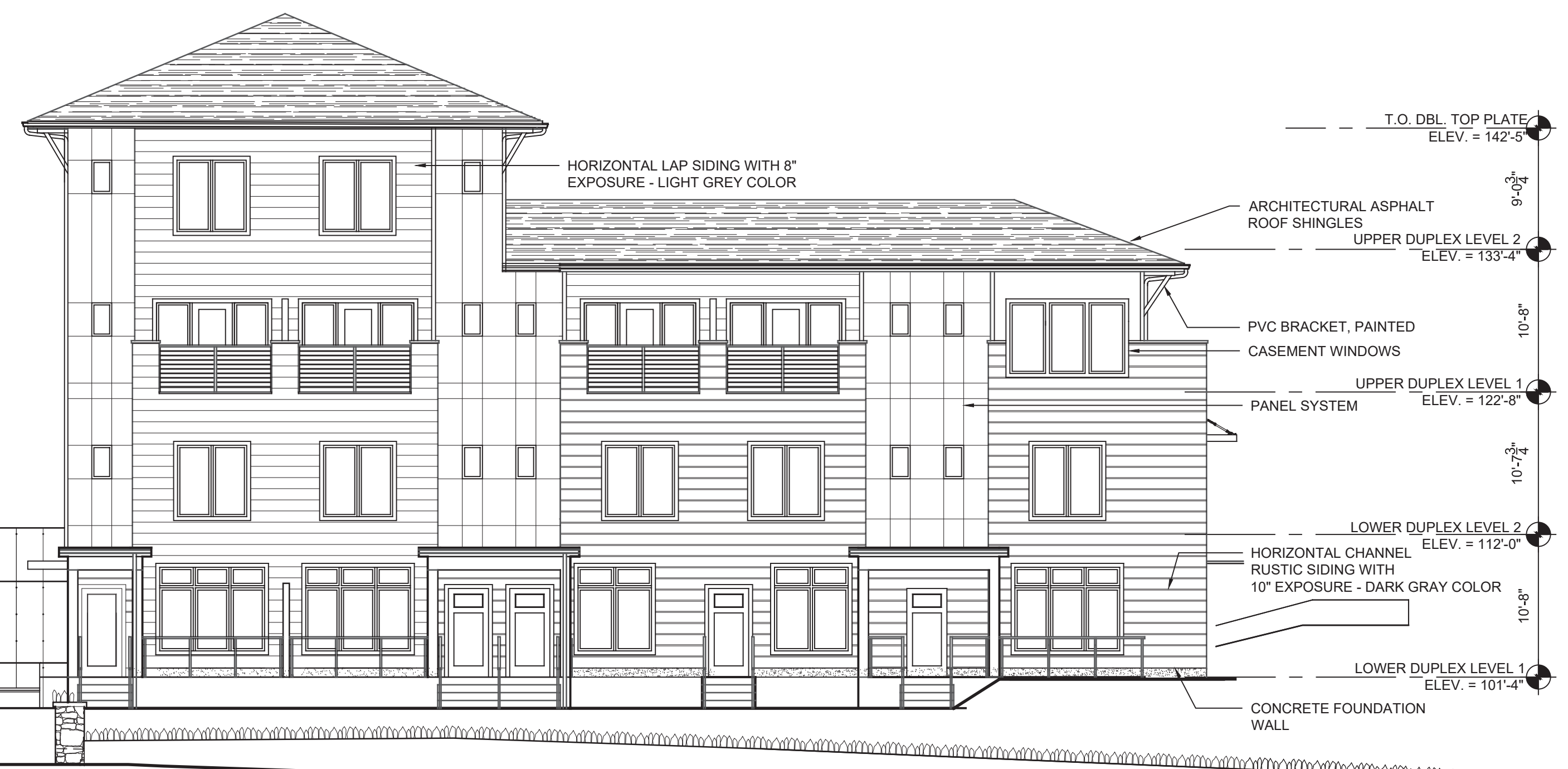
2 DONGAN BUILDING - NORTH ELEVATION (CURRENTLY APPROVED) 1/8" = 1'-0"
