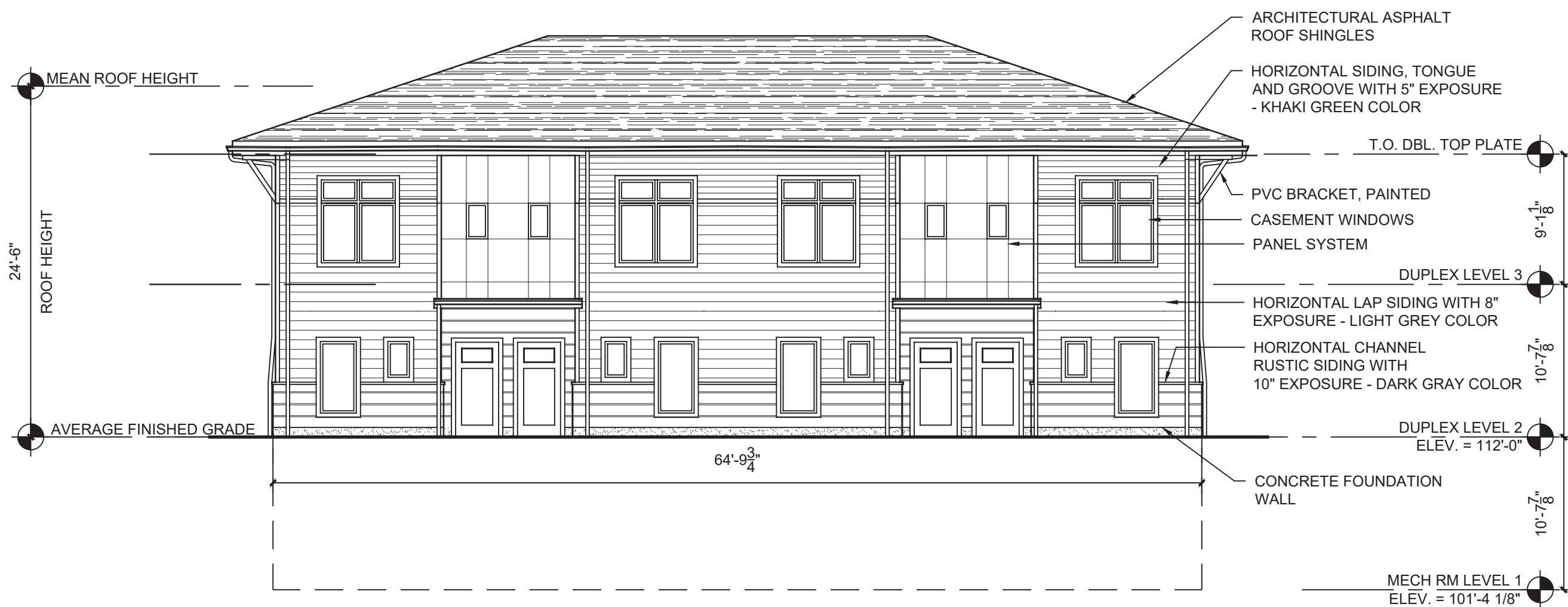
1 RIVER BUILDING - EAST ELEVATION (CURRENTLY APPROVED) 1/8" = 1'-0"
