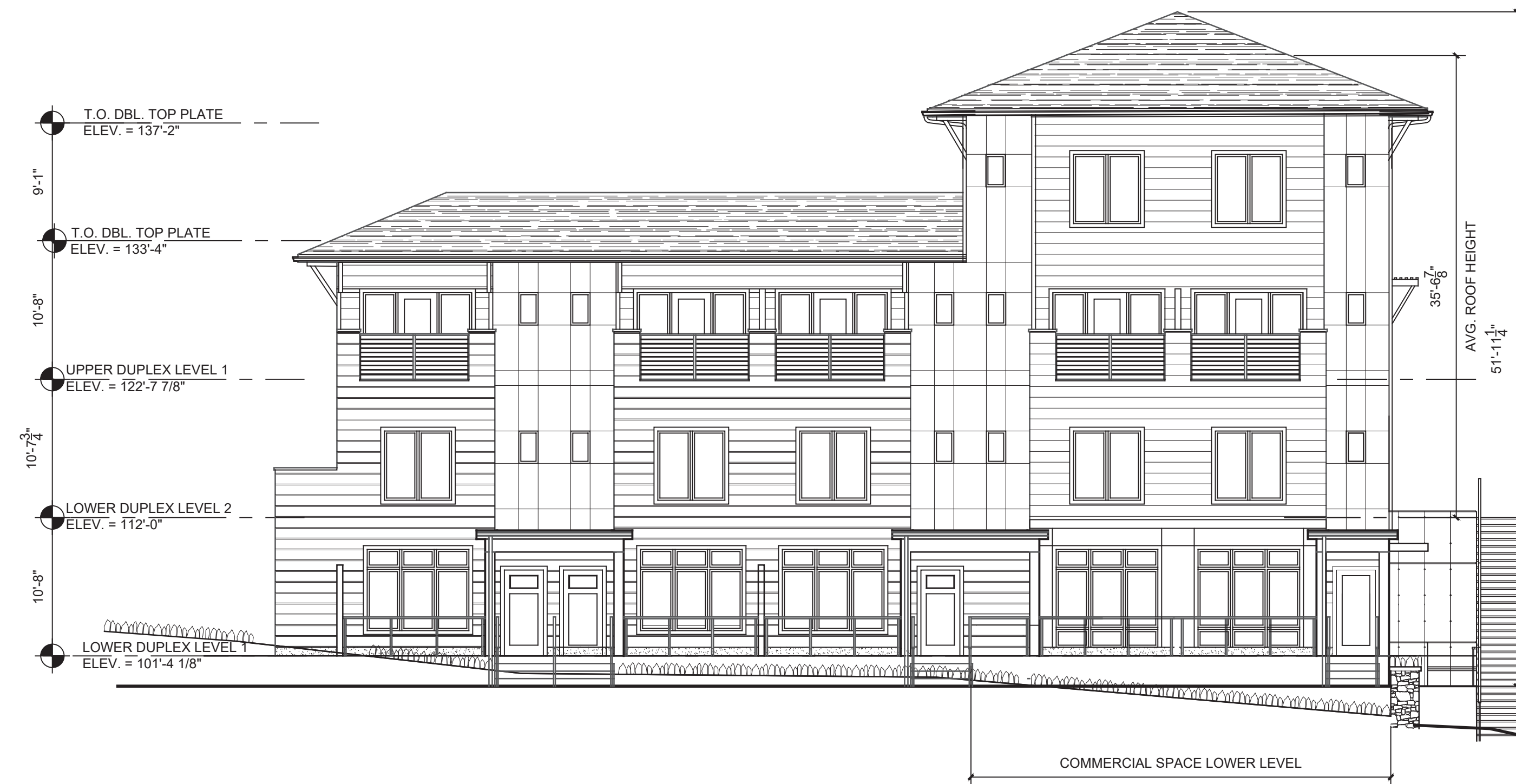
1 FALLKILL BUILDING - NORTH ELEVATION (PROPOSED) 1/8" = 1'-0"
