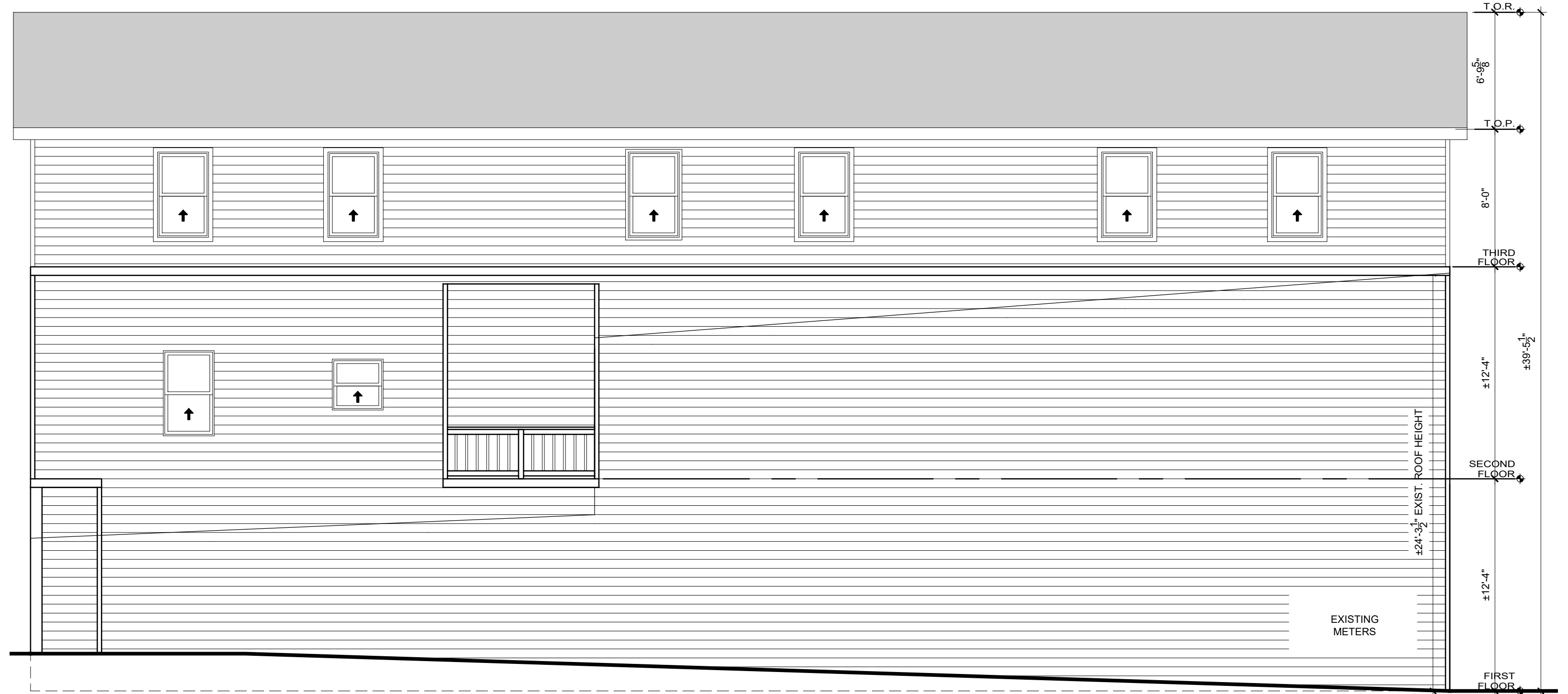
4 Existing & Proposed Left-Side Elevation (North Facing) ZB-2 Scale: 3/16" = 1'-0"
