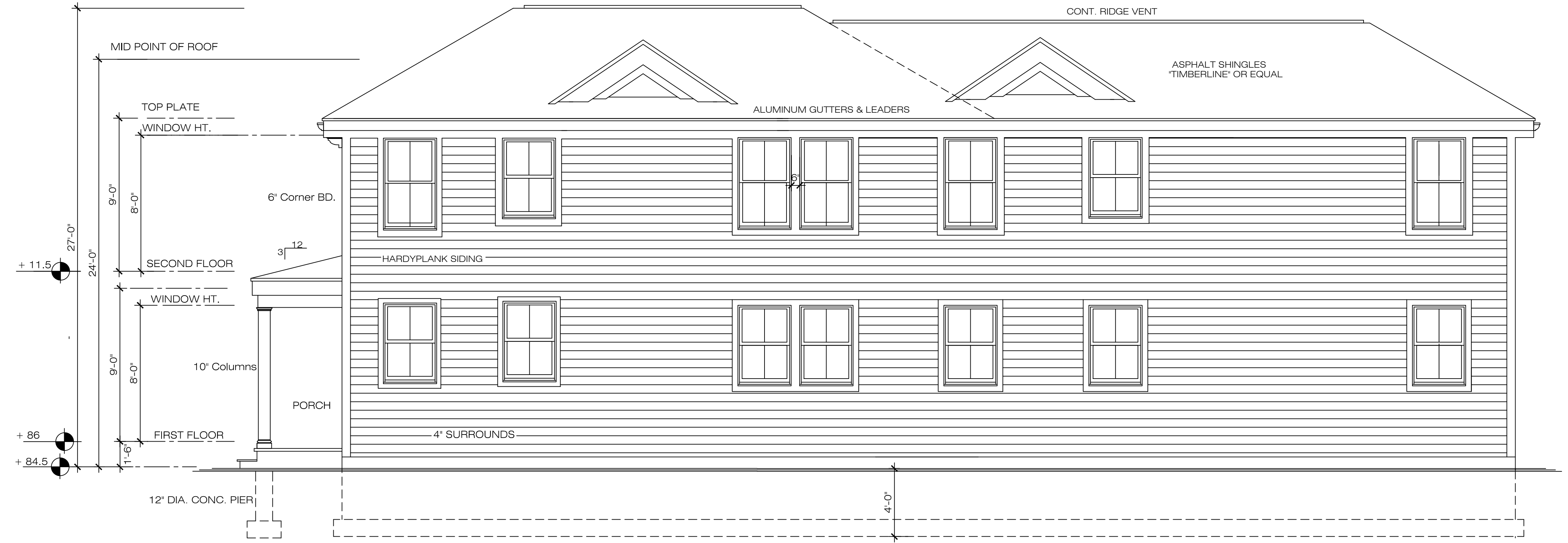
PROPOSED RIGHT ELEVATION SOUTH SCALE: 1/4" = 1'-0"
