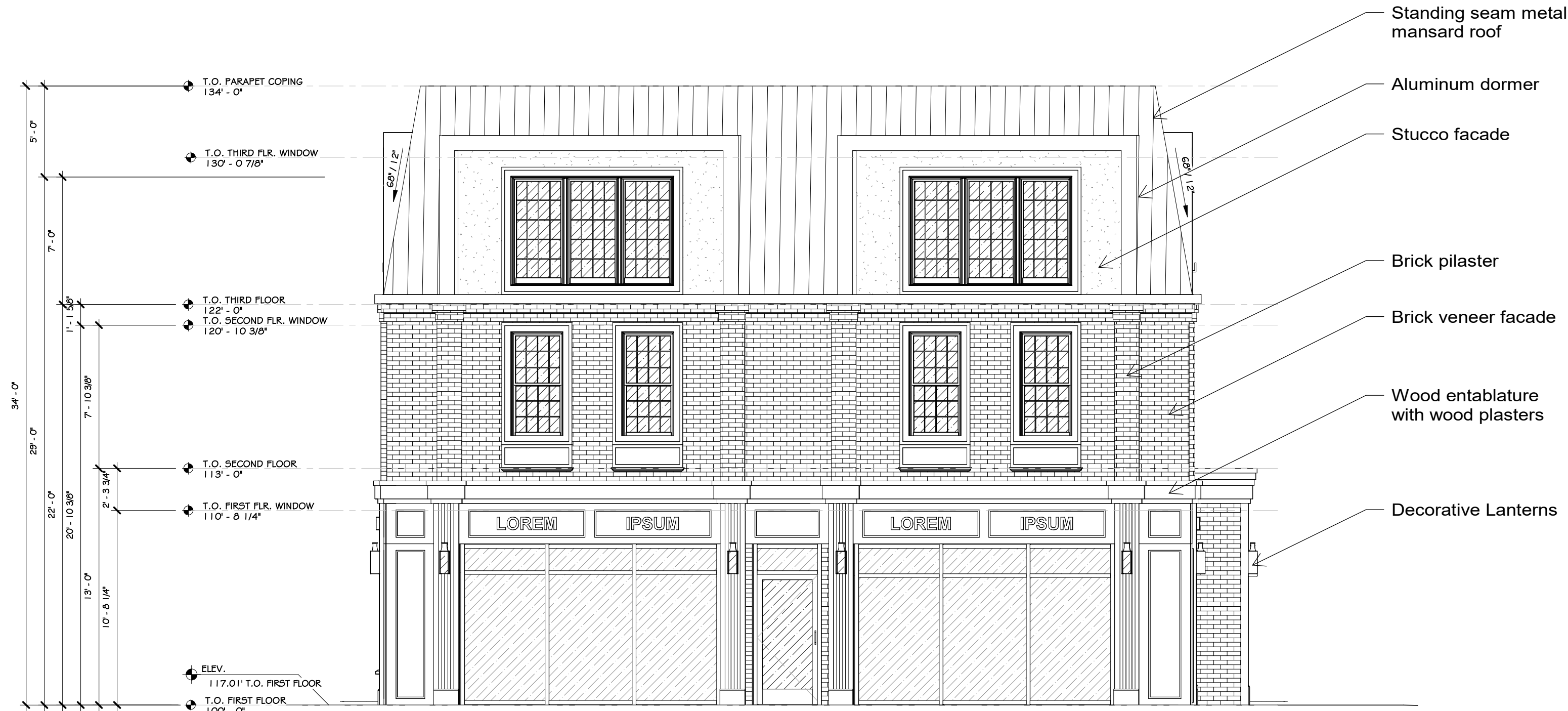
1 EAST EXTERIOR ELEVATION 3/16" = 1'-0"
