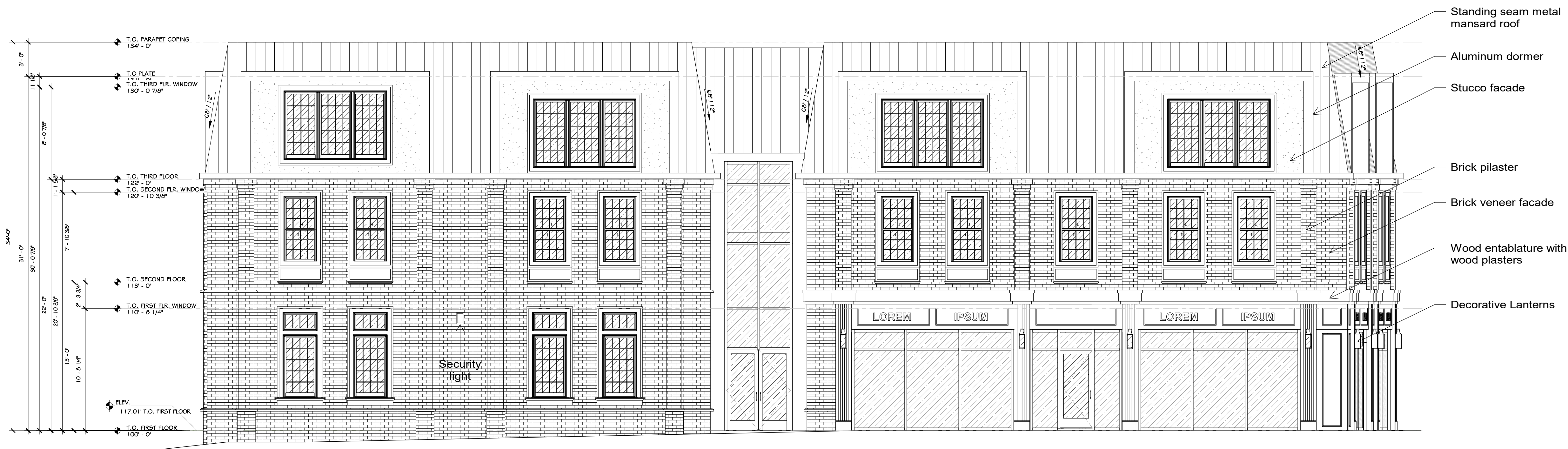
2 SOUTH EXTERIOR ELEVATION 3/16" = 1'-0"
