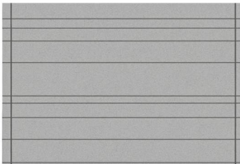
Exterior Facade: Manufacturer: Equitone Material: Fiber Cement Panel Color: BM Willow Creek 1468
