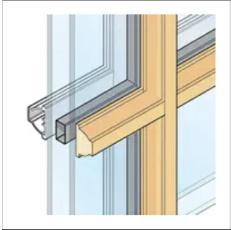
Pella "Integral Light Technology" ogee muntin profile with metal spacer
